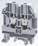
CHV6U 62 x 52 x 8 mm 0.2 - 6.0 mm 2 41 A, 1000 V, 0.8 Nm
