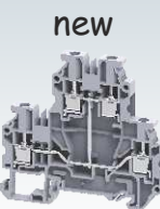
CYDL4(I.S) 65 x 70.5 x 6 mm 0.2 - 4.0 mm 2 32 A, 1000 V, 0.5 Nm
